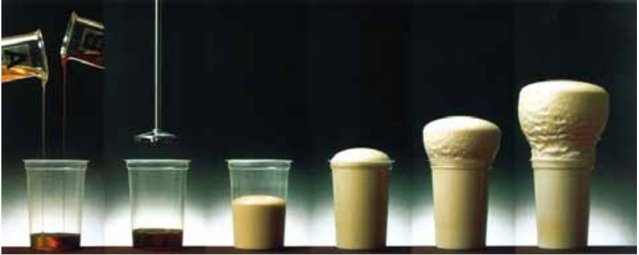
Figure 3. Blowing procedure of PU foam
